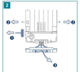
From the MLI Ultra, remove the Battery Safety Connector (1) and on either side the bolt closest to the positive terminal (2). Tilt the positive (right) side handle (3).
