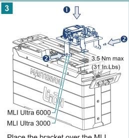
Place the bracket over the MLI Ultra (1), aligning the bracket holes with the holes of the bolts.
