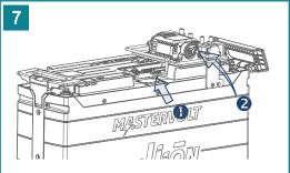
Put the Battery Safety Connector back in place (1).
