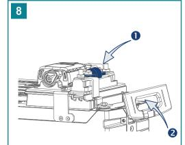
Remove the clear fuse cover and install the T-fuse (1). Place the cover back on the fuse holder. Close the side handle as much as possible (2). It will not close completely.
