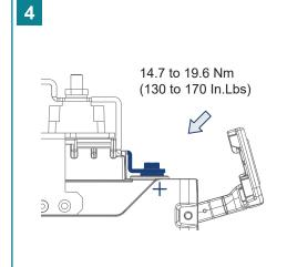
Secure the busbar conductor on the bracket to the positive terminal of the MLI Ultra.
