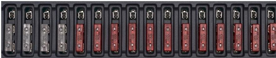
Figure 14. Fuses In Normal Operation
