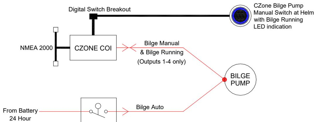
Figure 9. COI Bilge Pump Wiring Example
