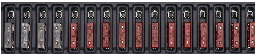
Figure 11. Fuses In Normal Operation
